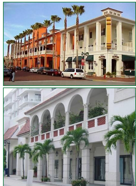
Figure 27. Examples of Façade Articulation
